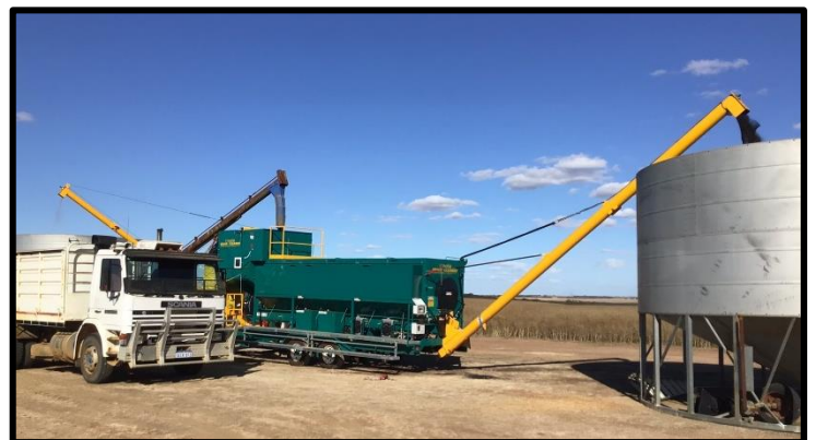
6 screen machine comes with a Yanmar 68kW (51hp) motor and a 230mm (9") clean grain auger. Rates to 50tph
