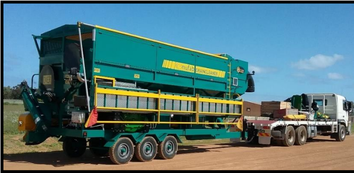
12 screen machine comes with a 140hp John Deere motor and a 330mm (13") clean grain auger.
